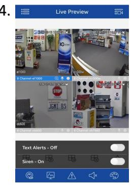
The default menu will be labeled as **Alarm Out 1** and **Alarm Out 2**. The siren should be wired into **Alarm Out 2** as illustrated by the "Siren - On" label in the figure above.
